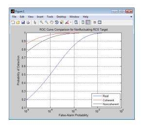
The ROC curves clearly demonstrate the superior probability of detection performance for coherent and noncoherent detectors over the real-valued case.
