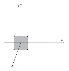
In the two preceding array geometries, the ULA and URA, the look directions of all the array elements are equal. In the case of the ULA, the *y*-axis is aligned with the array element apertures. This alignment is referred to as the *array axis*. The array elements have a common look direction, which the toolbox designates as the *x*-axis. As you can see, the *x*-axis is the direction orthogonal, or *normal* to the array axis.
