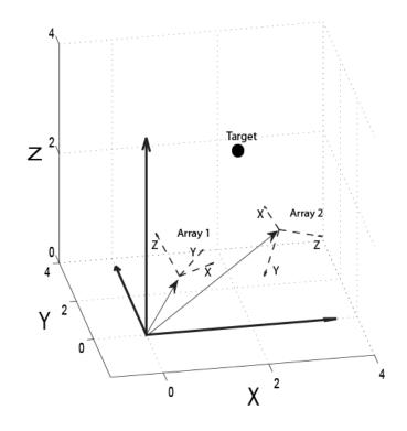
The two phased arrays detect the target and estimate target characteristics such as range and velocity. To translate information about the target derived from the two spatially-separated phased arrays, you must know the positions of the phased arrays and the orientation of their *local* coordinate axes with respect to the global coordinate system.
