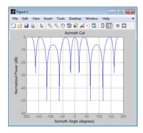
You can simulate the effects of phase shifts across your array using the collectPlaneWave method.
