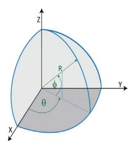
The azimuth angle is the angle between the positive x-axis and the orthogonal projection of the vector onto the xy plane. Angles from the positive x-axis toward the positive y-axis are positive angles and angles from the positive x-axis toward the negative y-axis are negative angles. The azimuth angle assumes values in the interval [-180,180] degrees.
