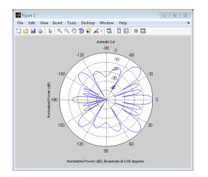
By default, plotResponse shows the array's normalized power response in decibels (dB) at zero degrees elevation for azimuth angles from [-180,180]. You can view azimuth cuts of the array response from various elevation angles and elevation cuts from various azimuth angles by specifying name-value pairs in plotResponse.
