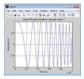
Use the step method to obtain your pulse waveform, and plot the real and imaginary parts of one pulse repetition interval.
