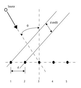
Because of the angle of arrival, the array elements are not simultaneously illuminated by the plane wave. The additional distance the incident wave travels between array elements is  $d \sin(\theta)$  where *d* is the distance between array elements. Therefore, the constant time delay between array elements is:
