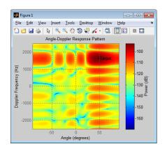
The angle-Doppler response shows the greatest response at 45 degrees azimuth and the expected Doppler shift.
