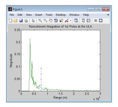
The large-magnitude clutter returns obscure the presence of the target. Apply the DPCA pulse canceller to reject the clutter.
