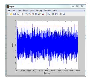
The red horizontal line in the plot is the threshold. You can see that very few sample values exceed the threshold. This result is expected because of the small false-alarm probability.
