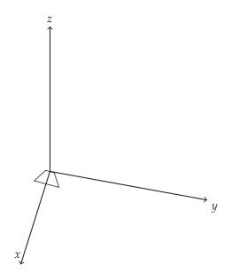
The figure shows the single array element located at the origin. For a number of array geometries, it is convenient to define the origin as the phase center of the array. For example, create a default uniform linear array (ULA) and query the element coordinates:
