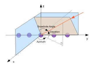
The shaded gray area in the figure is the plane determined by the signal incident direction and the array axis. The broadside angle is positive when measured toward the positive direction of the array axis. A number of algorithms for ULAs use the broadside angle instead of the azimuth and elevation angles. The algorithms do so because the broadside angle more accurately describes the ability to discern direction of arrival with this geometry.
