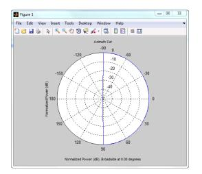
Use step to obtain the microphone's magnitude response at the specified azimuth angles and frequencies. The elevation angles are 0 degrees. Note the response is one at all azimuth angles and frequencies as expected.
