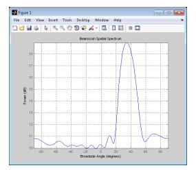
The beamscan estimator does not resolve the two sources based on their DOAs.
