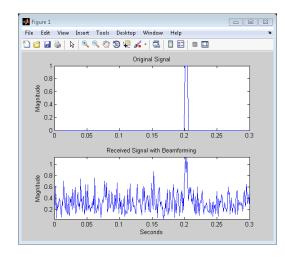
To examine the effect of the beamforming weights on the array response, plot the array normalized power response both with—and without—the beamforming weights.
