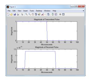
The delay in the received pulse is approximately 14  $\mu$ s, which is exactly what you expect for a distance of 4.123 km at the speed of light.
