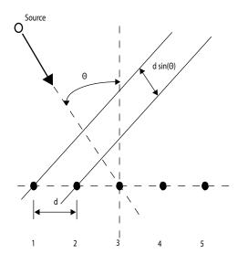
Assuming that the sensor frequency responses at the carrier frequency are identical, you can write the array transfer vector for the ULA as:
