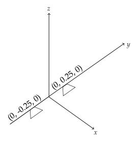
The elements are located 0.25 meters from the phase center of the array and the distance between the two elements is 0.5 meters.
