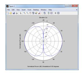
The antenna voltage response at zero degrees azimuth and 45 degrees elevation is cosd(45) as expected.
